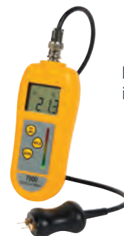
Measures moisture in concrete / hard floors
